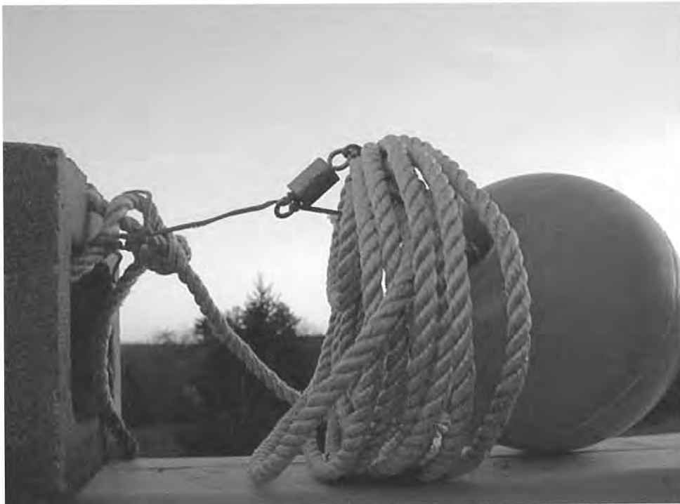
Galvanic time release link and associated hardware used in tests.
