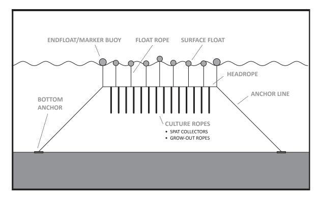
*Figure 7. Generalized diagram of an Icelandic mussel farming gear. Adapted from Gunnarsson et al., 2005. Source: author.*
