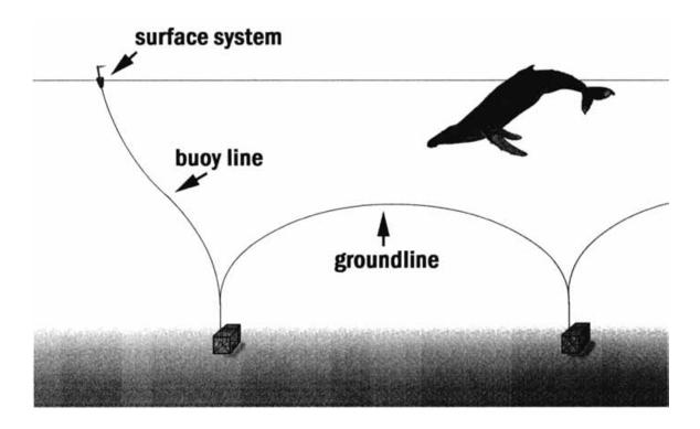
Figure 9. Generalized diagram of a pot gear and its associated parts, including groundline and buoy line. From Johnson et al., 2005. Copyright [2005] by the Society for Marine Mammalogy. Reprinted with permission.
