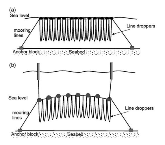
Figure 1. (a) Surface longline system (b) Submerged longline system. From Stevens et al., 2008. Copyright [2008] by Elsevier, B.V. Reprinted with permission.
