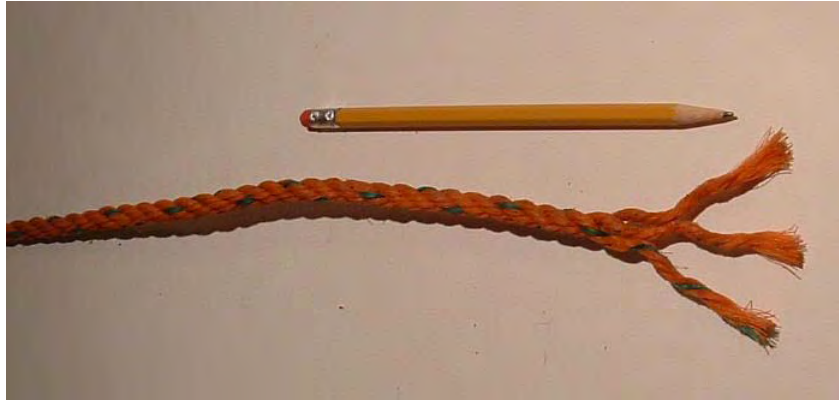
\frac{3}{8} inch orange PP 3-strand with green marker yarn- good condition.
