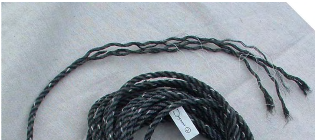
Frayed end may indicate tensile break
