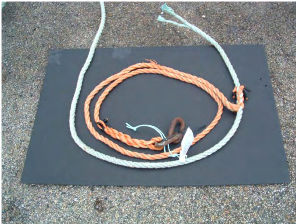
Connection of gangion. No specimen taken for gangion as it was so short.
