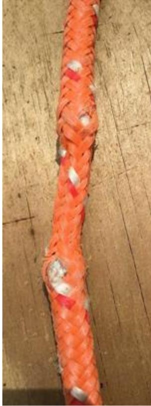
**Figure 12.** Post season braided sleeve shown with a gap and damage around ends of Everson (white) rope.
