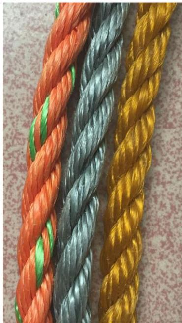
**Figure 1.** A piece of  $\frac{3}{8}$ -inch Manho-Manline float rope (left) with the two samples created at Taian Cord Rope of 2,425 lbf (middle) and 1,984 lbf (right).
