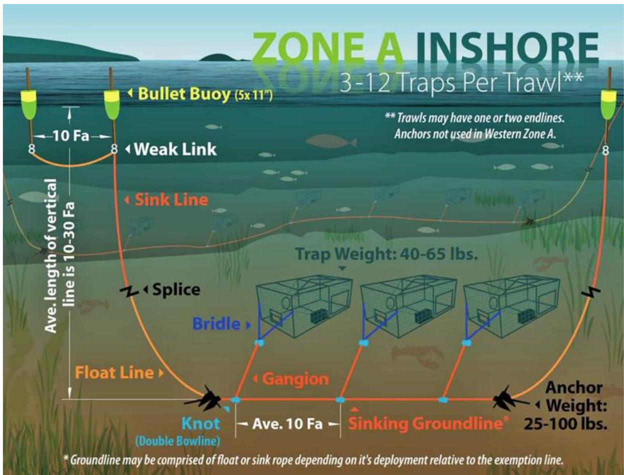
**Figure 25.** An illustration of a lobster gear configuration in the Gulf of Maine (Zone A Fishing Zone). There may be more than one endline (buoy line) on a lobster trawl, typically when the number of pots reaches five or more, but sometimes fewer. Fa = fathoms. (Illustration from McCarron and Tetreault, 2012).
