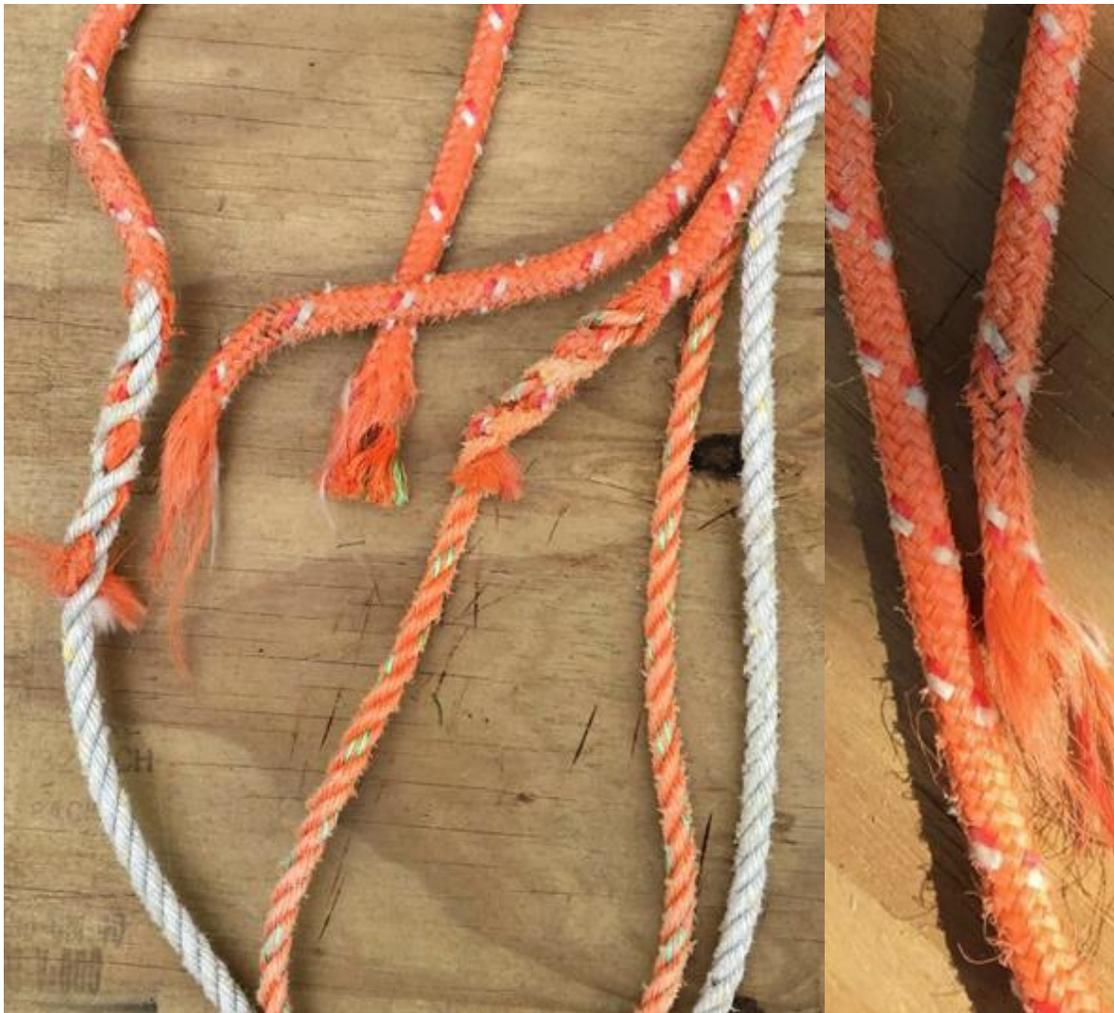
**Figure 11.** A Novabraid sleeve, Everson Pro and Manline rope with heavy abrasion. The sleeve was broken while hauling in the field (experimental break #7).
