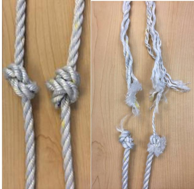
**Figure 7.** Single and double overhand knot in 3/8-inch Everson Pro rope before and after testing.
