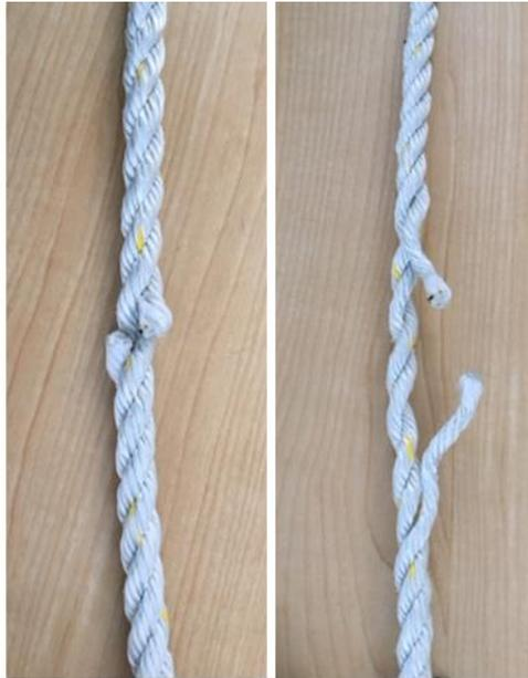
**Figure 6.** A 3-strand rope with a single strand cut before and after force was applied.
