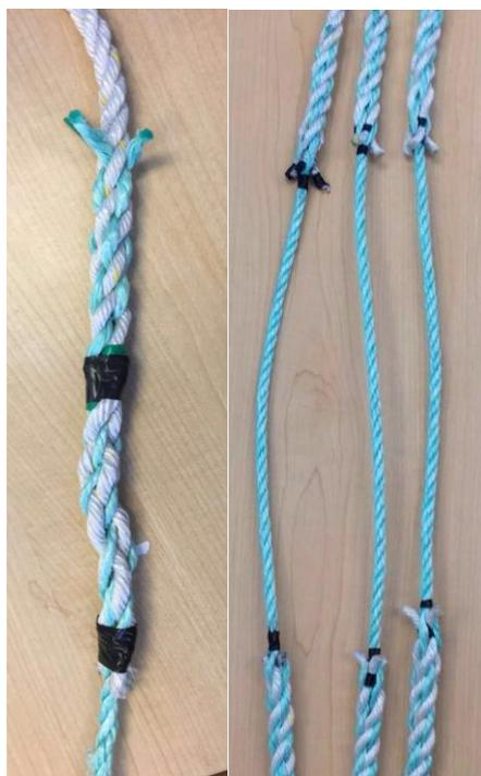
**Figure 5.** Spliced in 1/4-inch *Polysteel* design.
